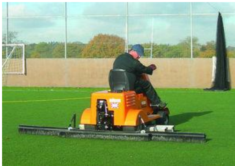
Ride-on brushing system with oscillating brushes
