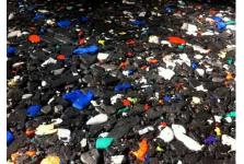
forms including polyurethane bound rubber mixes that are laid with a paving machine (often described as in-situ laid shock pads) or factory produced panels or rolls that are manufactured from a range of materials including rubber granules, polyurethane foam, expanded polyethylene beads and recycled polyethylene foam.
