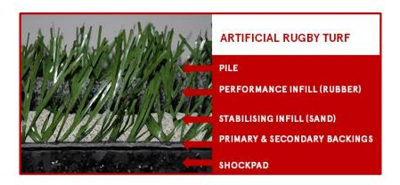
The surface comprises a long pile tufted carpet that is normally laid on a shock-absorbing pad that is laid on a free draining stone or macadam base. The pile of the carpet is partly filled with rubber granules to provide a cushioned surface that in conjunction with the shock pad underneath the carpet, provides the comfort and protection players require. Beneath the rubber granules is a layer of sand that provides weight to hold the carpet in place.
